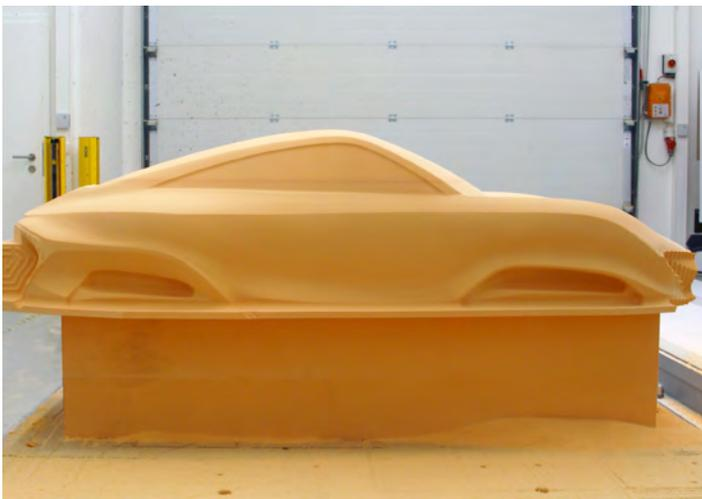
Fig.: The shape of the vehicle model is refined step by step in multiple milling passes.
