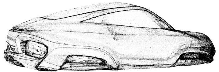
Fig.: Representation of the captured point cloud in PolyWorks
