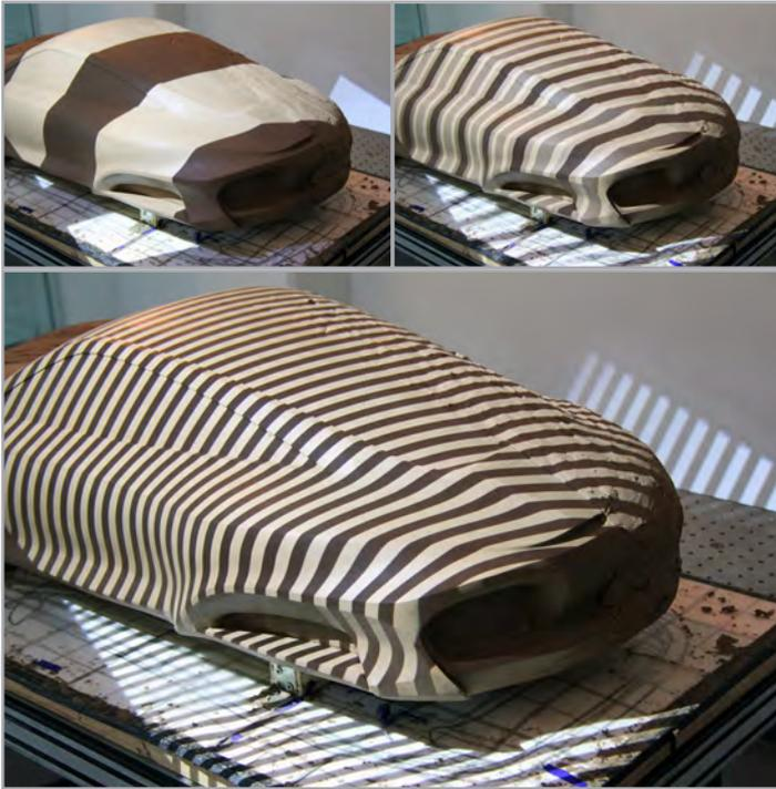
Fig.: A projector illuminates the measured object with patterns composed of parallel fringes of different widths and intensities.
