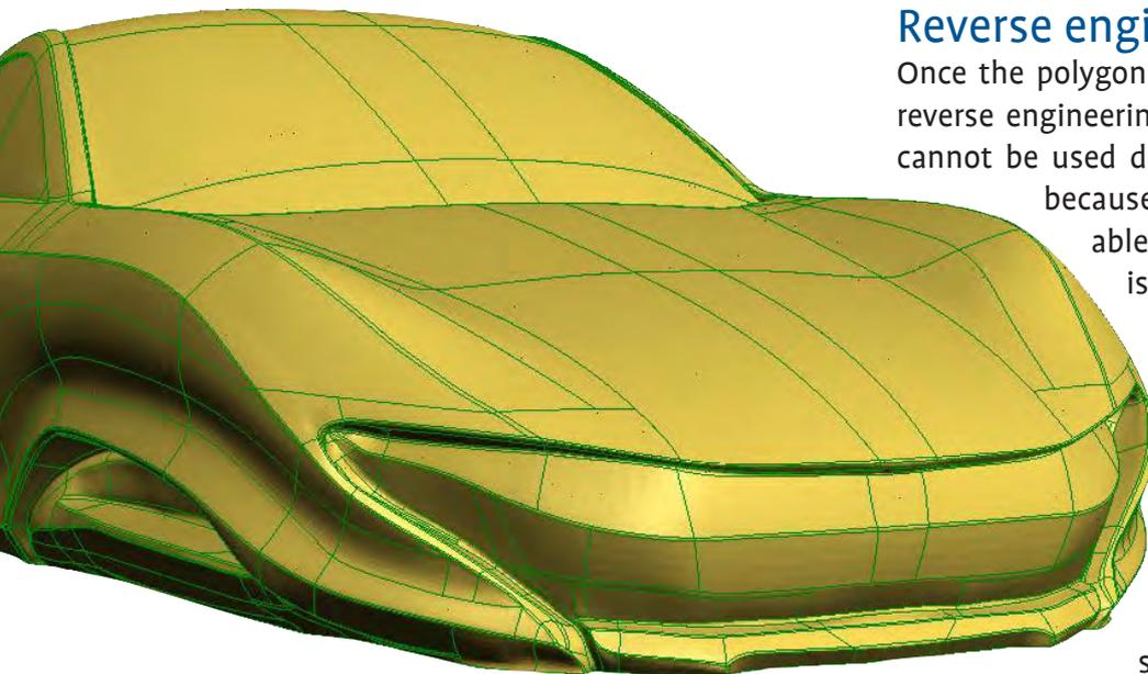
Fig.: The finished NURBS model consists of regular surface patches bounded by curves.
