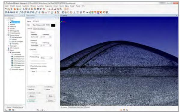
Fig.: In PolyWorks, closed triangle meshes are calculated from the point clouds.
